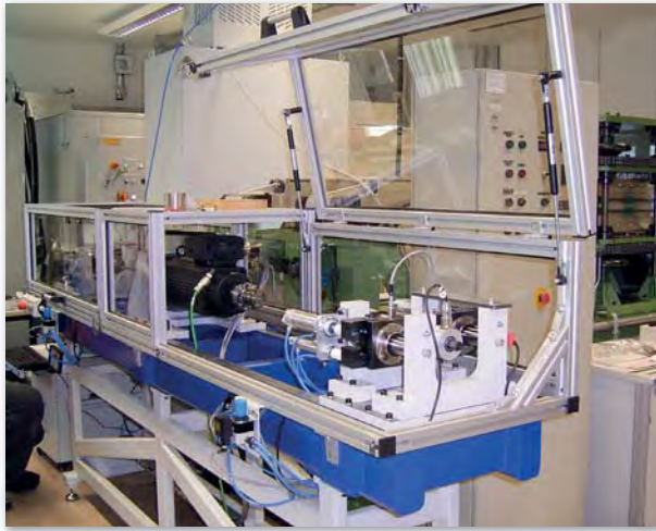
Torsion - Vibration Testing Machine 100 Nm, Test frequency 10 Hz
