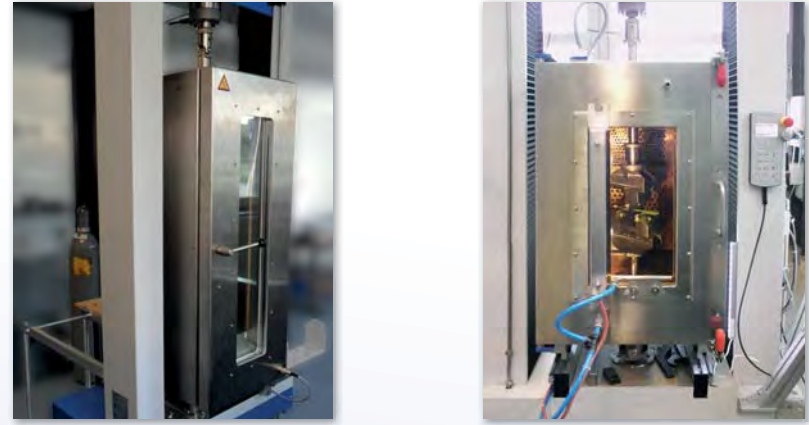
Climate chambers: temperature range -70 °C up to + 300 °C
