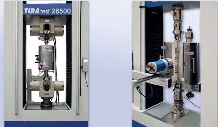
Hinged HT Furnaces are used for material testing under high temperature. · temperature range up to + 1200°C
